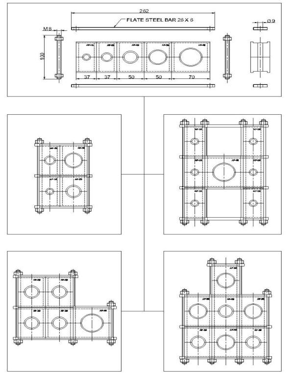
Due to the numerous stacking possibilities AIM PLAST does not carry accessories such as flat steel, threaded rods, nuts or sliding blocks in their product range!
